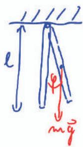
$$\text{NAUFR: } -mg \frac{l}{2} \cdot \sin \varphi = J \ddot{\varphi} \quad \begin{matrix} \bullet \sin \varphi \rightarrow \varphi \\ \bullet J = \frac{1}{3} ml^2 \end{matrix}$$
