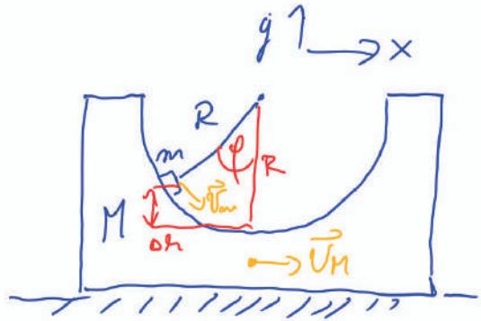
$$\begin{aligned} \bullet \Delta h &= R(1 - \cos \varphi) \approx R \frac{\varphi^2}{2} \\ \bullet G_x &= 0 \\ N_{mx} m + V_M \cdot M &= 0 \quad \varphi \rightarrow 0 \\ V_{mx} \downarrow &\quad V_M \downarrow \\ V_M &= -\frac{m}{M} V_{mx} \end{aligned}$$
