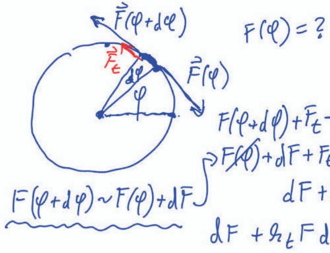
$$\begin{aligned} F(\varphi + d\varphi) + F_t - F(\varphi) &= 0 \\ F(\varphi) + dF + F_t - F(\varphi) &= 0 \\ dF + F_t &= 0 \\ dF + h_t F d\varphi &= 0 \end{aligned}$$
