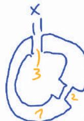
$$H_1 = \frac{NI}{2\pi r + l(\frac{S_1}{S_2} - 1) + x \frac{S_1}{S_2} (\mu - 1)}, B_1 = \mu \mu_0 H_1$$
