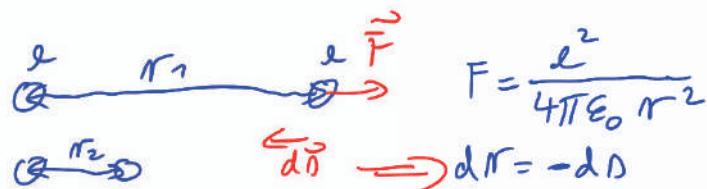
$$A = \int_{r_1}^{r_2} \vec{F} \cdot d\vec{s} = \int_{r_1}^{r_2} \frac{l^2}{4\pi\epsilon_0 r^2} dr = \frac{-l^2}{4\pi\epsilon_0} \left( -\frac{1}{r} \right) \Big|_{r_1}^{r_2} =$$
