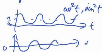
$$\Rightarrow \underline{\underline{dW_{AVG(t)}}} = \frac{m}{\ell} \omega^2 u_0^2 \left( \frac{1}{2} \cos^2 \omega x + \frac{1}{2} \sin^2 \omega x \right) dx \\ = \frac{1}{2} \frac{m}{\ell} \omega^2 u_0^2 dx$$
