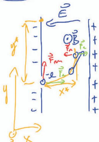
$$\vec{F} = q(\vec{E} + \vec{v} \times \vec{B}) \Rightarrow m \begin{pmatrix} \dot{x} \\ \dot{y} \\ \dot{z} \end{pmatrix} = q \begin{pmatrix} -E_x \\ 0 \\ VB \end{pmatrix} = q \vec{E} + q(\vec{v} \times \vec{B})$$
