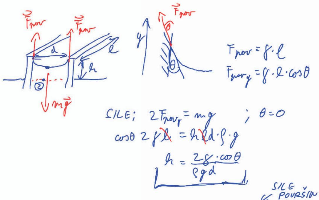
$$\text{TLAK: } \Delta p_{\text{norm}} = \frac{2 \gamma \cdot l \cos \theta}{d l}$$
