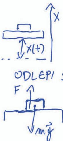
$$\begin{aligned} x &= x_0 \sin(\omega t) \\ \dot{x} &= \omega x_0 \cos(\omega t) \\ \ddot{x} &= -\omega^2 x_0 \sin(\omega t) = -\omega^2 x \end{aligned}$$
