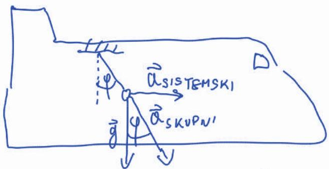
$$tg \varphi = \frac{a_{\text{sistemski}}}{g} = \frac{0,7}{10} \rightarrow \underline{\varphi = 4,1^\circ}$$
