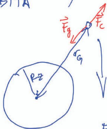
SATELIT JE VES ČAS NAD ISTO TU ČKO  $\Rightarrow \omega = \omega_z = 2\pi/V = \frac{2\pi}{T_0}$ ;  $T_0 = 1 \text{ dan}$
