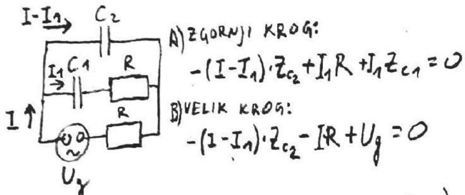
$$(12A) I = \frac{I_1}{Z_{C_2}} \left( Z_{C_2} + R + Z_{C_1} \right) = I_1 \left( 1 + \frac{R}{Z_{C_2}} + \frac{Z_{C_1}}{Z_{C_2}} \right)$$
