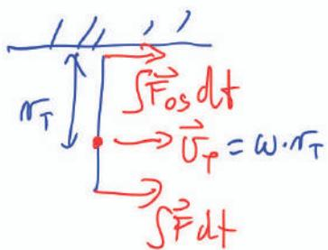
$$4mV_T = \int \vec{F}_{\text{os}} dt + \int \vec{F}_{\text{fd}} dt = mv_0$$
