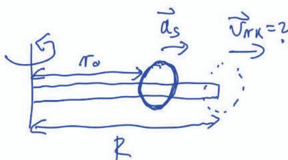
$$\bullet \vec{a}_s = \omega^2 \vec{r} \quad "V_r"$$
