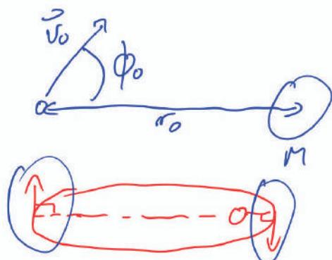
$$T: m V_0 r_0 \cdot \sin \phi_0 = m V_1 r_1$$
