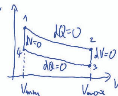
$$1 \rightarrow 2: dQ_{12} = 0 \quad T_1 V_1^{\gamma-1} = T_2 V_2^{\gamma-1} \Rightarrow T_2 = T_1 \left( \frac{V_1}{V_2} \right)^{\gamma-1} < T_1$$
