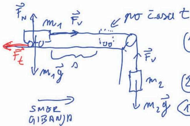
$$\begin{aligned} (1) \quad & F_v - F_t = m_1 a \\ & F_N - m_1 g = 0 \end{aligned}$$
