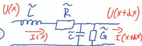
$$\tilde{G} = \frac{dG}{dx} \leftarrow \begin{array}{l} \text{PREVODNOST} \\ \text{DIELEKTRIKA} \end{array} \quad \boxed{\frac{1}{\epsilon_0}}$$
