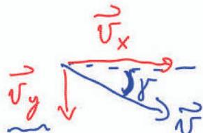
$$\text{HITROST: } v_x = v_0 \cdot \cos \beta = 20 \text{ m/s} \cdot \frac{1}{2} = 10 \text{ m/s}$$
