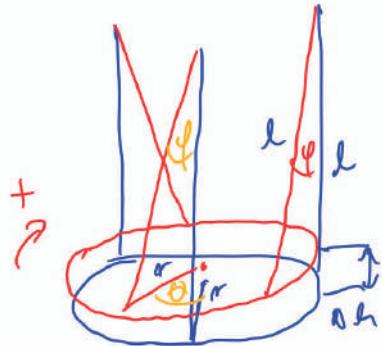
$$\Delta h = l(1 - \cos \varphi) \xrightarrow{\varphi \rightarrow 0} l \frac{\varphi^2}{2} \quad \cos \varphi \approx 1 - \frac{\varphi^2}{2}$$
