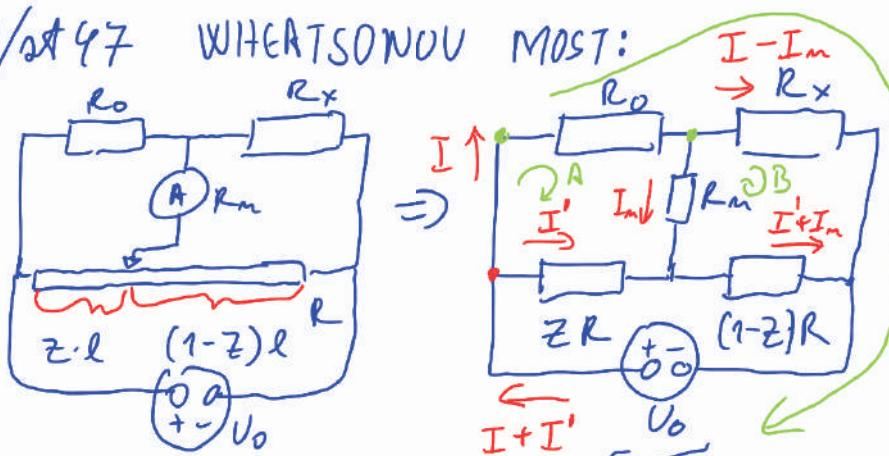
$$\bullet I_m [(1-z):z = 3:7] = ? \quad A: -IR_o - I_m R_m + I' z \cdot R = 0 \Rightarrow I' = \frac{IR_o + I_m R_m}{zR}$$
