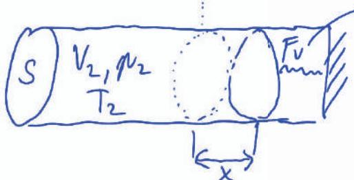
$$V_2 = V_1 + S \cdot x$$
