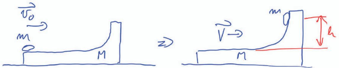
$$\text{a) W: } \frac{\gamma h V_0^2}{2} = mgh \Rightarrow h = \frac{V_0^2}{2g} = 0.2 \text{ m}$$
