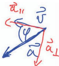
$$\vec{r} = (x, y) = (A \cos \omega t, B \sin \omega t); \omega = \frac{2\pi}{t_0}$$
