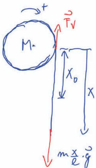
$$\text{SILE: } m \frac{x}{l} g - F_V = m \frac{x}{l} \alpha \Rightarrow F_V = m \frac{x}{l} (g - \alpha)$$
