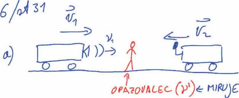
$$v' = v_1 \frac{1}{1 - \frac{v_1}{c}}$$
