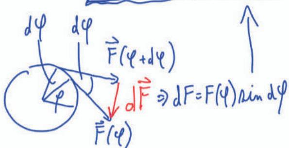
$$\begin{aligned} dF &= -h_t F d\varphi \\ \int_{F_0}^{F_1} \frac{dF}{F} &= -h_t \int_0^{\varphi_1} d\varphi \\ \ln \frac{F_1}{F_0} &= -h_t \varphi_1 \\ F_1 &= F_0 e^{-h_t \varphi_1} \end{aligned}$$
