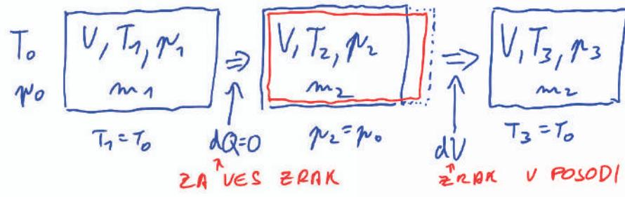
$$1 \rightarrow 2: dQ=0; \quad \rho_1^{1-\gamma} T_1^{\gamma} = \rho_2^{1-\gamma} T_2^{\gamma}$$
