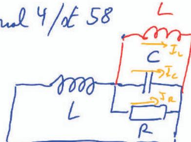
$$U_L = U_C = U_R \quad ; \quad U_C = Z_C \cdot I_C = i\omega C I_C$$
