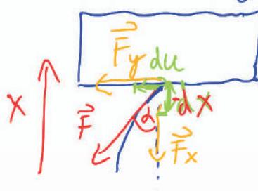
$$\begin{aligned} F_y &= F \sin \alpha = -F \left( \frac{du}{dx} \right) \\ \operatorname{tg} \alpha &= \frac{du}{dx} \end{aligned}$$
