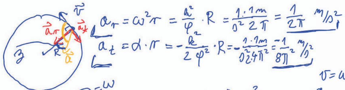
$$a_r = \omega^2 r = \frac{\dot{\varphi}^2}{\varphi^2} \cdot R = \frac{1 \cdot 1 \text{ m}}{0^2 2\pi} = \frac{1}{2\pi} \text{ m/s}^2$$
