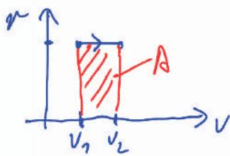
$$\bullet A = - \int_{V_1}^{V_2} p dV = - p(V_2 - V_1) = - \underline{\underline{200J}}$$
