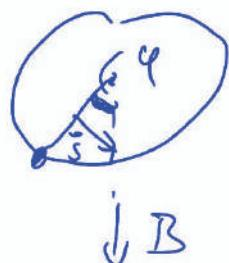
$$\begin{aligned} S &= \pi R^2 \\ \vec{B} \cdot \vec{S} &= B \cdot S \sin\varphi \\ &= B R^2 \sin\omega t \end{aligned}$$
