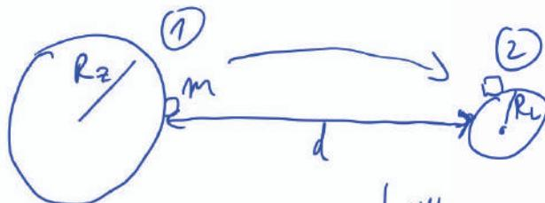
$$A = \Delta W_p = W_{p2} - W_{p1} \quad \left| \begin{array}{l} W_{p1} = -\frac{\mathcal{J} M_Z m}{R_Z} - \frac{\mathcal{J} M_L m}{R_L + d} \\ W_{p2} = -\frac{\mathcal{J} M_Z m}{R_Z + d} - \frac{\mathcal{J} M_L m}{R_L} \end{array} \right.$$
