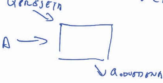
$$\begin{aligned} \eta_C &= \frac{|Q_{reject}|}{|A|} = \frac{T_{Nizja}}{T_{Visja} - T_{Nizja}} = \frac{1}{\eta_C(\text{TOPLOINR})} \\ &= \frac{1}{1 - \frac{T_{Nizja}}{T_{Visja}}} \end{aligned}$$
