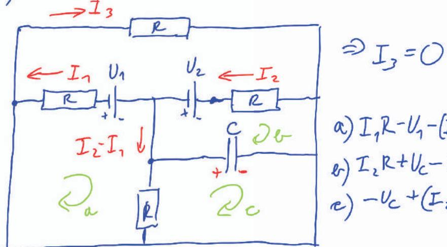
$$\begin{aligned} a) I_1 R - U_1 - (I_2 - I_1)R &= 0 \\ b) I_2 R + U_c - U_2 &= 0 \\ c) -U_c + (I_2 - I_1)R &= 0 \end{aligned}$$
