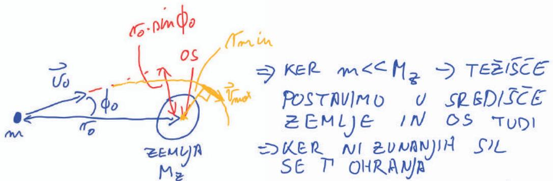
$$\Gamma: \gamma h V_0 \cdot r_0 \sin \phi_0 = \gamma h V_{\max} r_{\min} \Rightarrow V_{\max} = V_0 \frac{r_0 \sin \phi_0}{r_{\min}}$$
